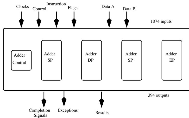
Fig. 1.2 Adder Units Inside of `fadd`
